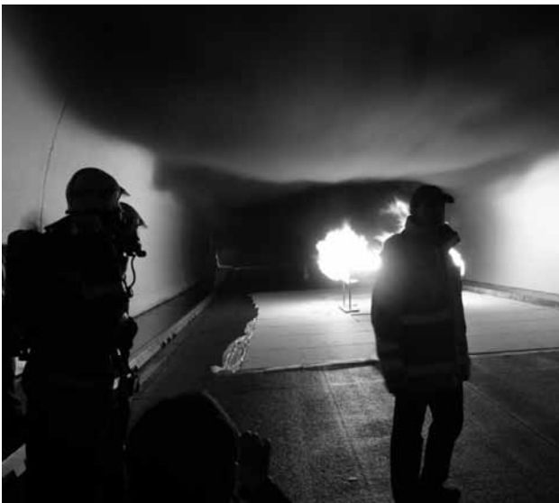
Fire testing of the smoke control system in the 2.4km long Kirchdorf S35 Tunnel (20km north of Graz, Austria), May 2010, just prior to opening.
