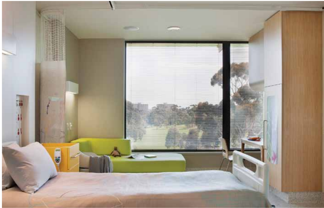
This patient room has two functional areas that can be separated via a curtain screen. The room has good access to daylight. Individual control has been provided to each area so that separate light levels can be achieved in bed and lounge areas. Ambient and reading lighting is supplied from luminaires located behind the bed. Downlights provide supplementary task lighting as required.
